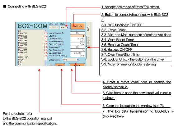
Setup example> If you change a value in the setup window (see 4. above), its Corresponding value in the window (see 3. above) will be changed; the data in the BLG-BC2 will be changed accordingly and automatically.
