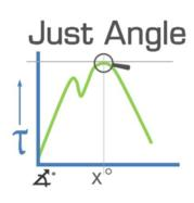
In Just Angle Mode, the maximum torque reading will remain on the OLED display when the load is removed as long as the torque loaded is above the 10% of maximum capacity threshold. The angle turned from 5% of the tool span until maximum torque reading is also displayed. The user has the option to store the reading in memory. If storage of the reading is not required, the user may continue to the next measuring task.
