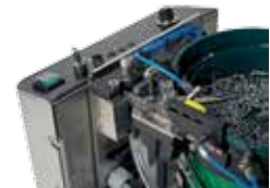
Selector adjustment to increase or decrease speed of cycle
