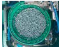
Vibrating Bowl with special coating to grip screws
