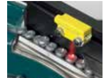
Optical Sensor prevents screws from getting jammed in the selection track
