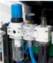
Filter and lubrication unit with compressed air pressure gauge. Lubricator for use with pneumatic drivers only
